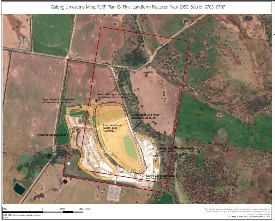
Figure 3 Final landform and rehabilitation plan - Final landform features
