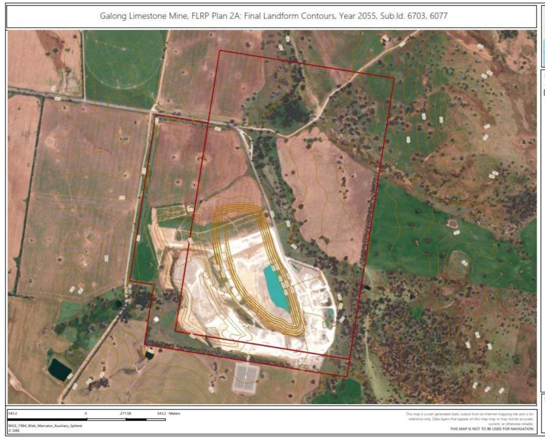
Figure 5 Final landform and rehabilitation plan - Final landform contours
